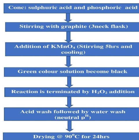
Fig.2. Preparation of graphene oxide by modified hummer method
